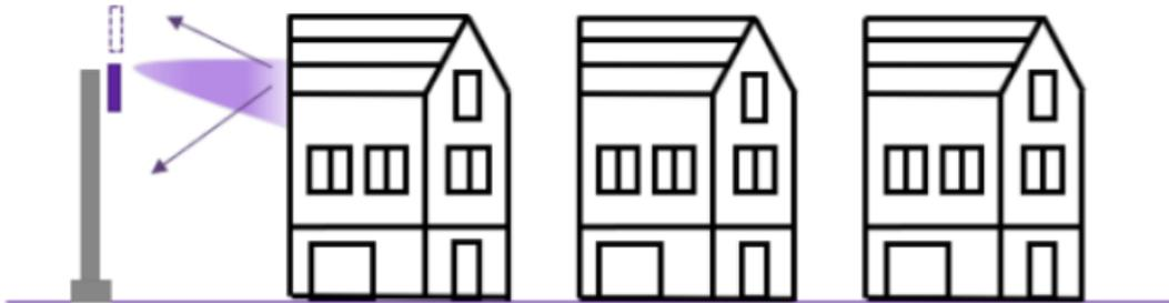
The ideal height for mobile antennas is 5m taller than surrounding buildings and obstructions, with space for additional antennas used for sharing the mast and growth.
