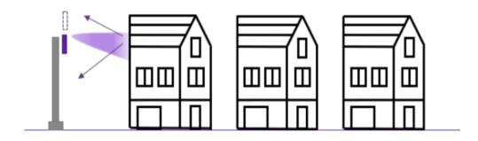
The ideal height for mobile antennas is 5m taller than surrounding buildings and obstructions, with space for additional antennas used for sharing the mast and growth.
